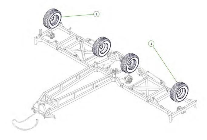
All wheel nuts tightened to 305Nm
