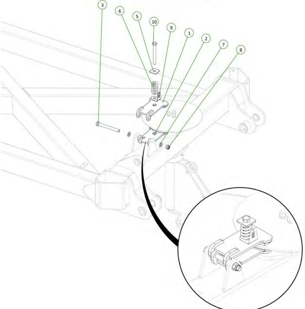
Check tension of brake caliper spring (50-63mm road transport)
