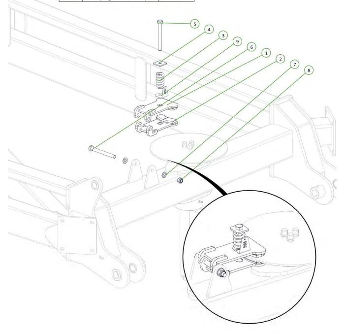
Check tension of brake calliper spring (50-63mm road transport)
