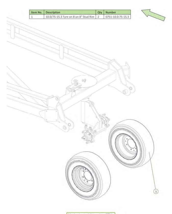
All wheel nuts tightened to 125Nm
