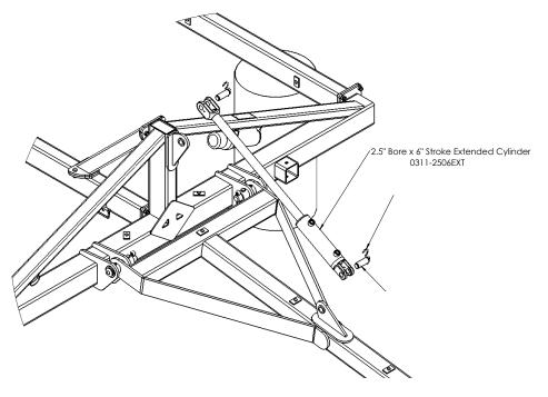
A flow reducing orifice needs to be fitted to the extend (base) end of the Hitch cylinder to prevent sudden movement when operating the levelling cylinder.
