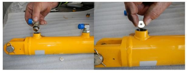
Remove the 8UNO to 8JIC elbow from the extend port.
