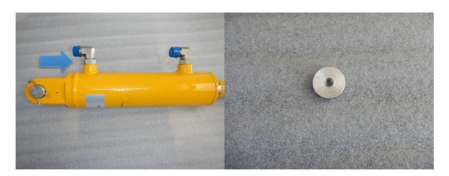
Before installing the cylinder. Part no. 0311-2506EXT, an orifice 8UNO-RES-FIX-2 must be fitted to the extend port.
