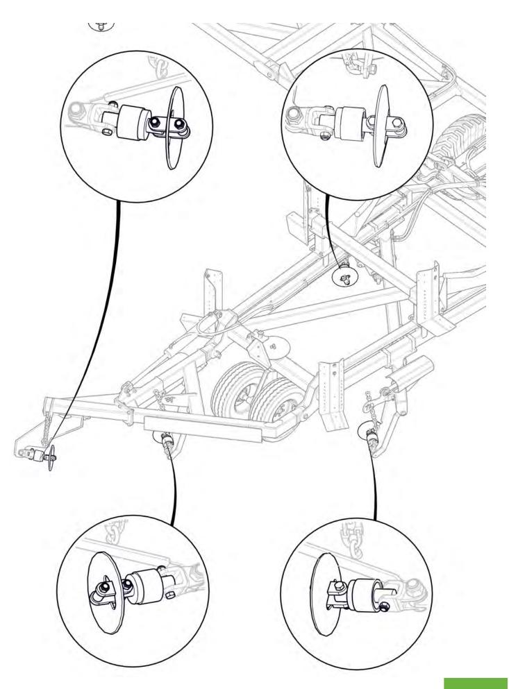
All bearings correctly orientated with seal facing the rear of the machine
