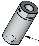
0343-924001261 1/2" BSPP 60 micron inline filter max flow 60L/M & 5000psi max pressure
