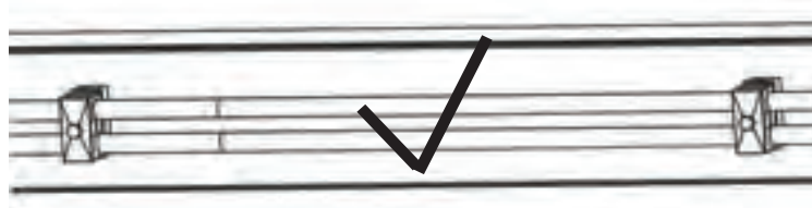
Correct layout of hoses
