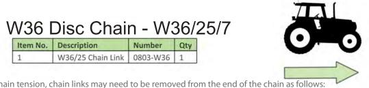
For correct chain tension, chain links may need to be removed from the end of the chain as follows: W36 Disc Chain - cut a disc chain link from the end of the disc chain
