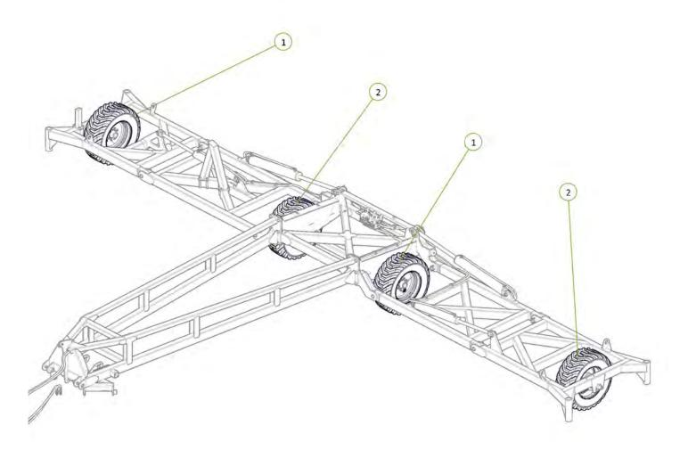
All wheel nuts tightened to 100ft-lb / 140Nm
