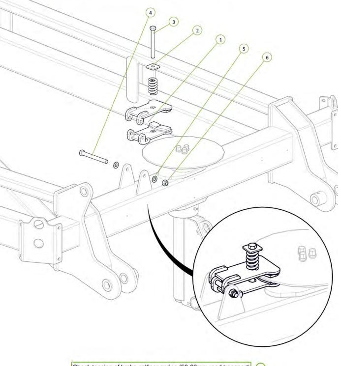
Check tension of brake calliper spring (50-63mm road transport)
