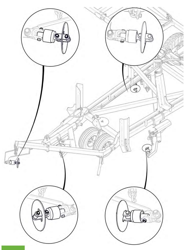
All bearings correctly orientated with seal facing the rear of the machine
