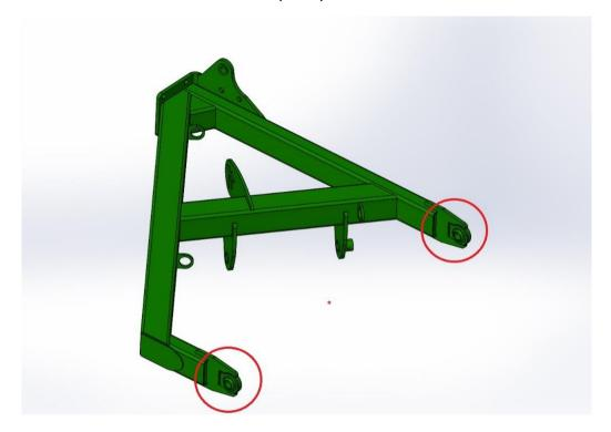
Swivel balls added to rear A-frame pivot points
