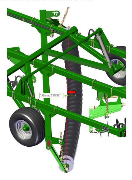
Indicator line shows acceptable curvature when operating.
