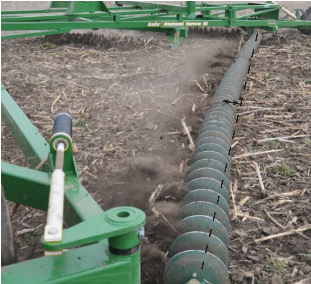
Indicator line shows acceptable curvature when operating
