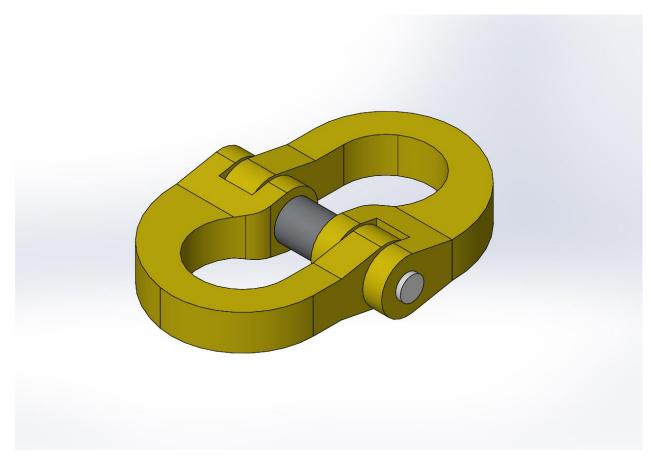
Components with a higher load rating (part number 0801-CMAH13N) have therefore been issued to replace the affected links. Each machine has 8 links which require replacement as shown in the schematic below.
