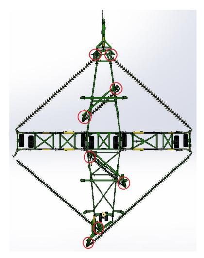
The height adjustment chains should be removed from the machine in order to facilitate replacement of the link. The old component should be held securely in a vise and disassembled by knocking out the pin using a punch. The replacement component should be re-assembled in the same manner, with the chains then being re-assembled onto the machine.
