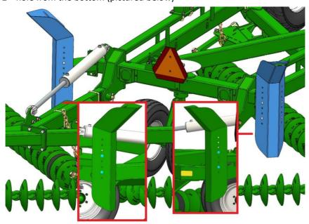
12. Remove and DISCARD the highlighted pipe guard from the tail.
