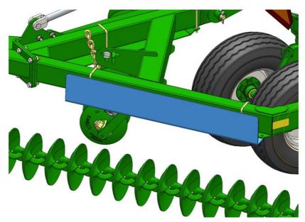
14. Fold the machine, ensuring chain does not snag or catch and sits securely ready for transport. The chain management upgrade is now complete. [NOTE: Ensure that chains are correctly tensioned as per the Operators Manual. Failure to do so can lead to premature chain wear, incorrect machine folding and warranty being void]
