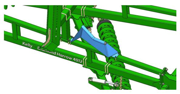
6. Remove and set aside the highlighted chain carrier ends, then remove and DISCARD the chain carrier beam and pedestals from the rear A-Frame.
