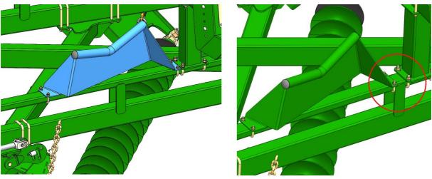
10. Attach the 0810-162 outrigger extensions to the back corners of the machine using the supplied coach head bolts and supplied 0271-16162129U u-bolts.
