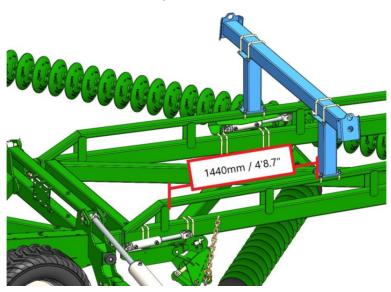
8. Re-mount the chain carrier ends onto the chain carrier beam at the height settings pictured below.
