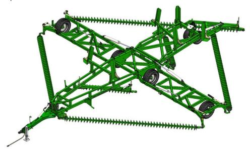
2. Remove and set aside the chain carrier ends, then remove and DISCARD the front outriggers and chain carrier beam from the front A-frame (highlighted components).
