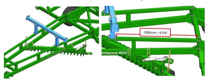
4. Re-mount the chain carrier ends onto the chain carrier beam with the lowest bolt in the 3<sup>rd</sup> hole from the bottom as pictured.
