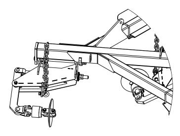
Step 2: Remove rear tension box by removing the pivot pin and sdjustor chain
