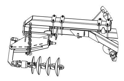
The machine is now ready to be used. This kit adds 3 chain links to the RHR chain allowing more overlap at the rear of the machine.
