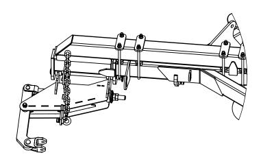
Step 6: Lock the pivot pin into position using the Locking bush (0810-RFTT-LC) supplied as shown below
