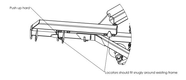
Step 4: Using the U-Bolts and plates supplied clamp the fram into position as shown below
