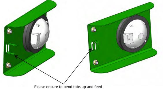
Please ensure to bend tabs up and feed wire through, so the light cable is secure
