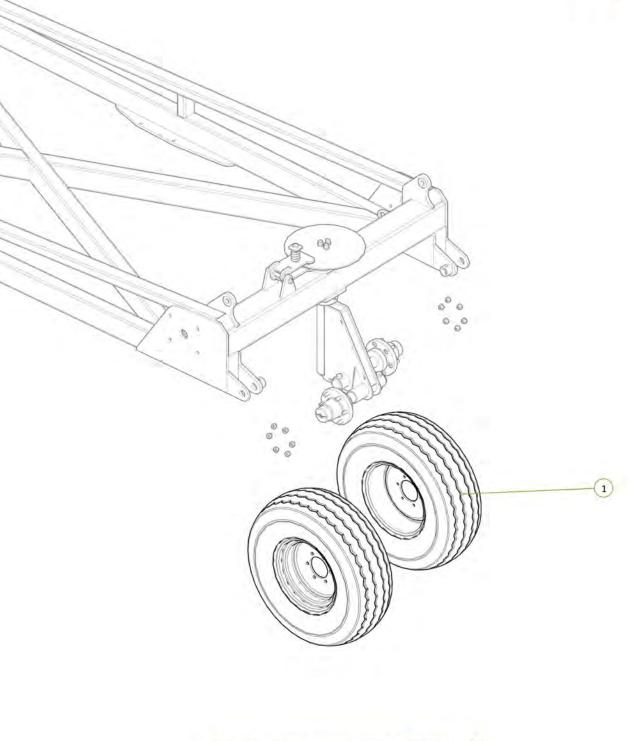
All wheel nuts tightened to 90ft-lb / 125nm
