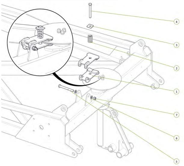
Check tension of brake caliper spring (50-63mm road transport)
