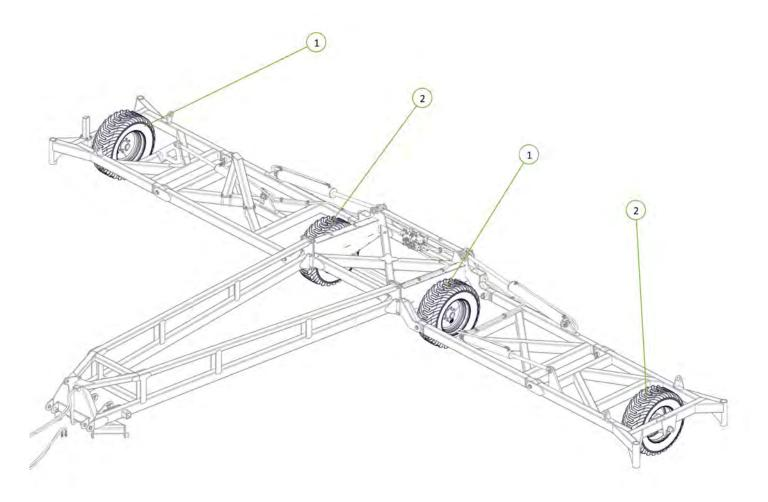
All wheel nuts tightened to 100ft-lb / 140Nm
