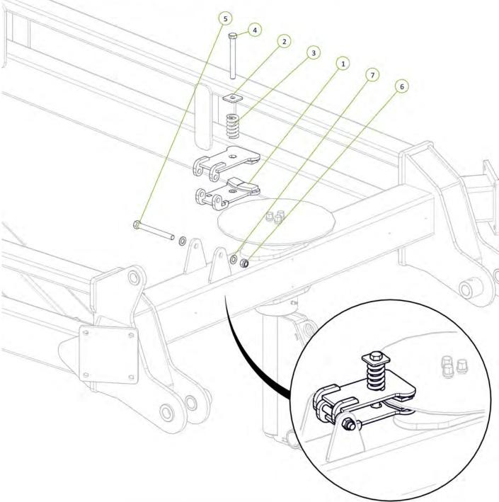
Check tension of brake calliper spring (50-63mm road transport)
