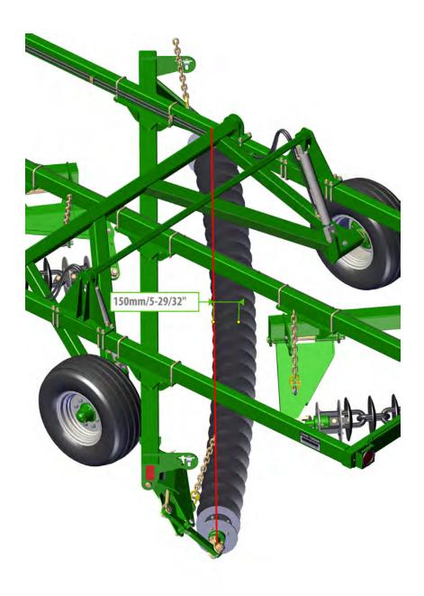
Indicator line shows acceptable curvature when operating.
