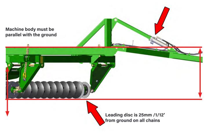
Check the length of the height adjusting chains on the two front chain mount plates. There should be no slack in the chain and about 25-51mm /1/12'-1/6' of gap between the ground and the bottom of the first disc machine near the centre line.
