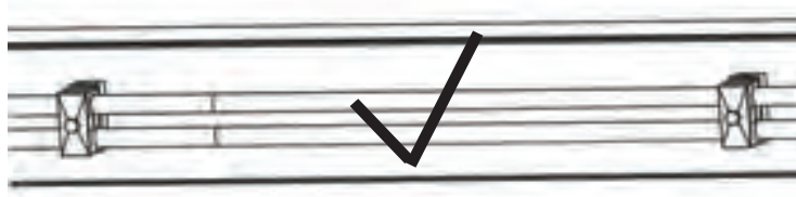
Correct layout of hoses
