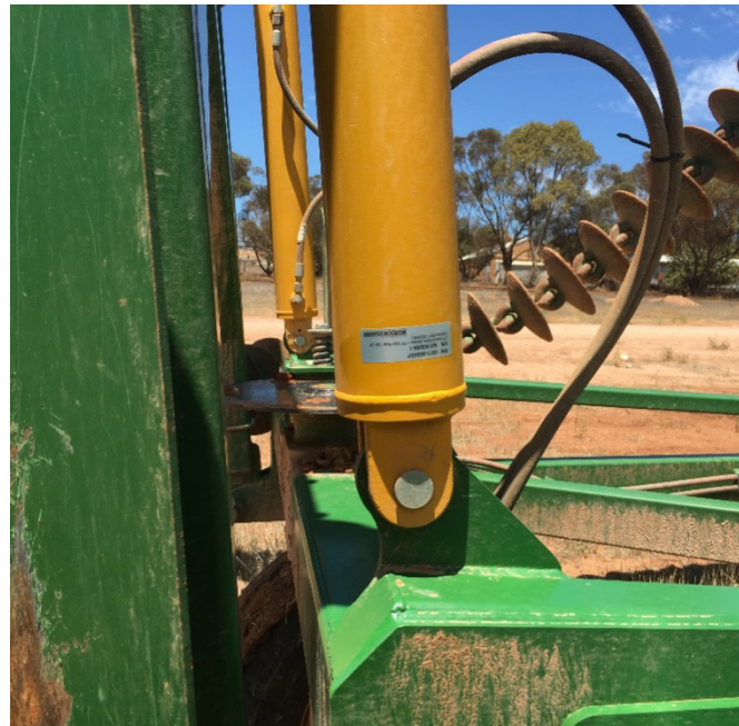
[LEFT] an Ezyfit cylinder (0311-2958) with the stamping on the barrel clevis. [CENTRE] Nordon cylinder (0311-3524SP) with sticker on barrel. [RIGHT] white Nordon cylinders
