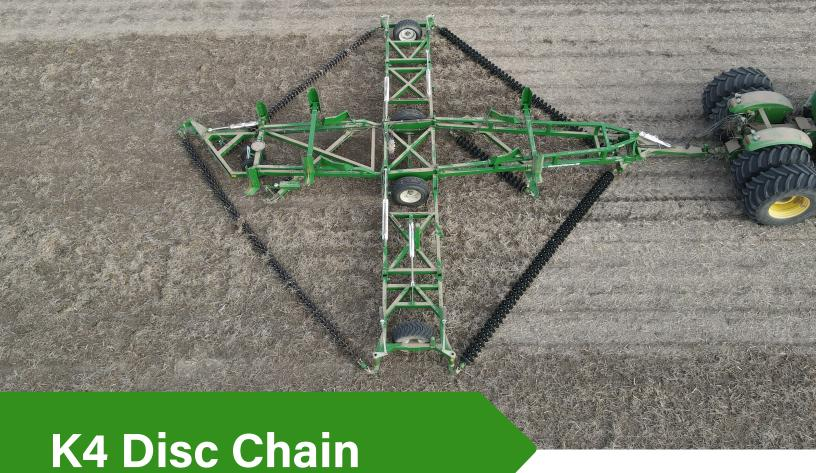
The K4 Disc Chain is a new disc specifically designed for enhanced weed control in a broad range of soil types. This disc sits between the heavy, more aggressive CL2 Disc Chain and the versatile CL1. The K4 combines the benefits of a replaceable bladed disc with the efficiency of a lightweight build and closer disc spacing.
