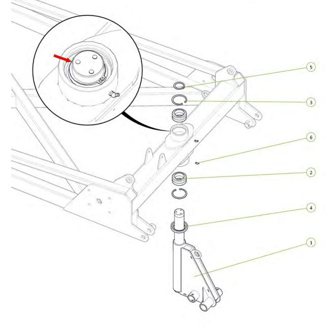
Circlip fitted to Jockey Wheel shaft
