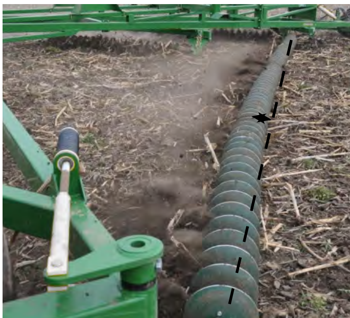
Indicator line shows acceptable curvature when operating
