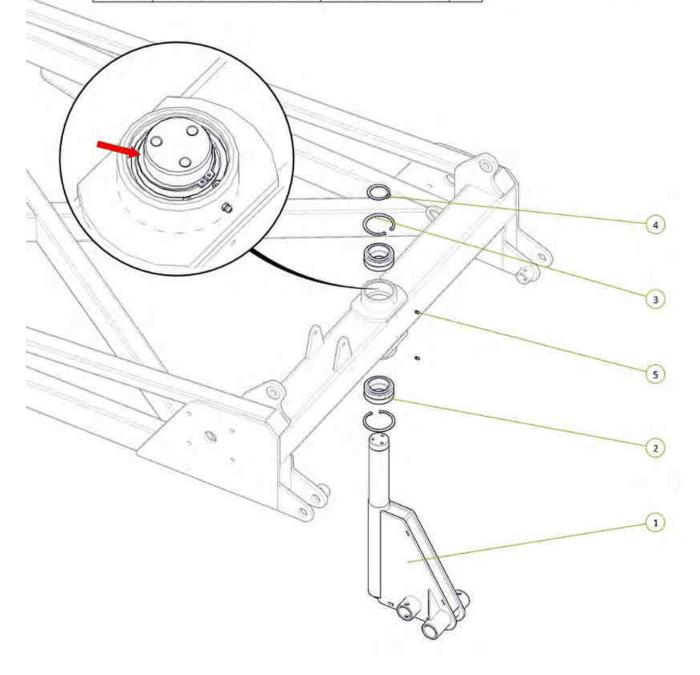
Circlip fitted to Jockey Wheel shaft
