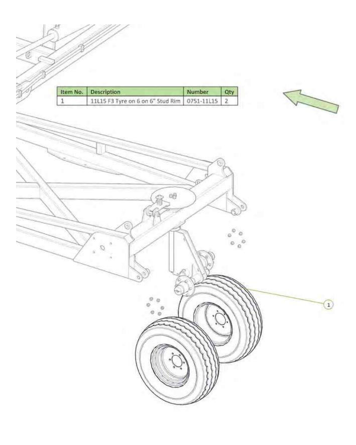
All wheel nuts tightened to 90ft-lb / 125Nm
