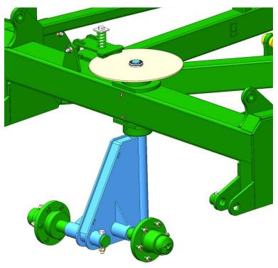
Tighten in a cross pattern, Bring all bolts up equally to 17Nm (12.54 Ft/Lbs) (caution if a single bolt is done up to tension there is a risk of the bolt breaking)
