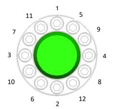
To undo, remove all bolts and gently tap collar with a hammer and collar should become loose.
