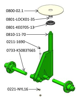
Slide shaft of jockey wheel up through both bearings.
