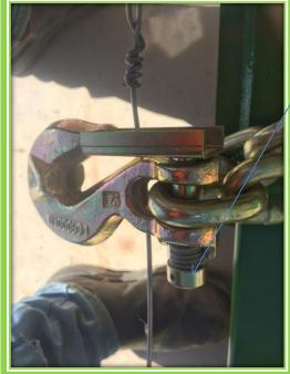
Ensure hook is being assembled as seen in picture with the collar on the opposite side to the hook.
