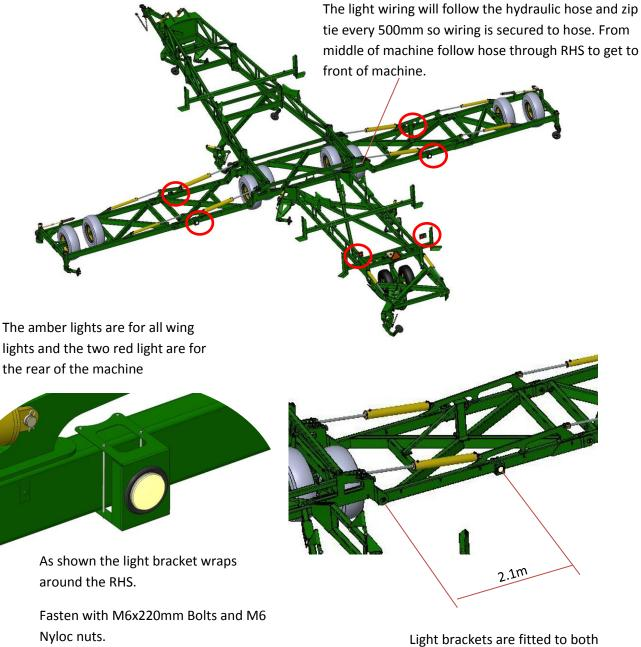
Light brackets are fitted to both front and rear of machines 2.1m in from the pivot pin, as shown here.
