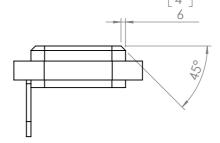
**STEP 10:** Set up and re weld the cut off section to the base of the rear drop leg tube as shown below.
