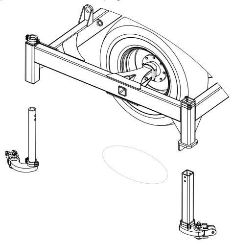
**STEP 4:** With the droplegs removed lower the wing frame back to ground level as shown below
