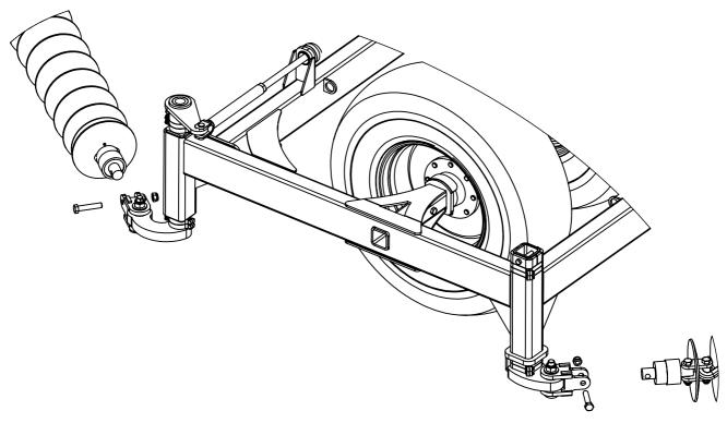
**STEP 2:** Remove the front chain tension assembly and the rear drop leg retaining plates as shown below
