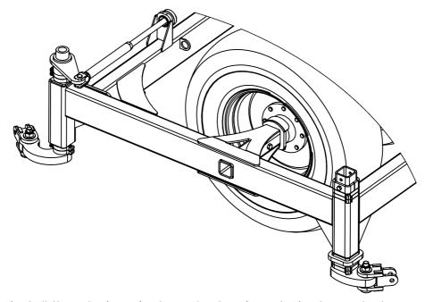
**STEP 13:** Reinstall the chain swivels and retension chain shown below.
