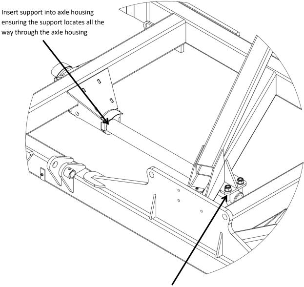
Using u bolt clamp up end of axle support to provide pre load to axle beam
