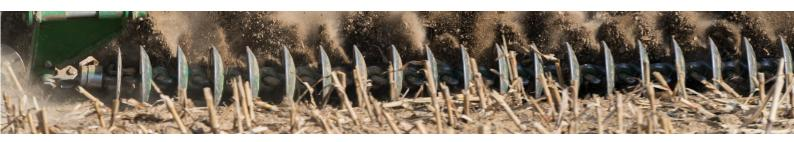
Properly managing residue after harvest is crucial for providing the best environment for your next crop. Shallow-working tillage technology can mulch and incorporate residues in one pass, saving time and energy. Kelly Disc Chains break stubble and split internodes to accelerate biological decomposition, leaving an insulating mulch layer and returning nutrients to the seedbed. Strong, fast and efficient: the Kelly Tillage System is the ultimate tool for residue management.
