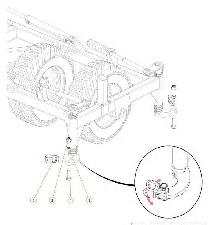
Ensure ALL clevis's can pivot after installation
