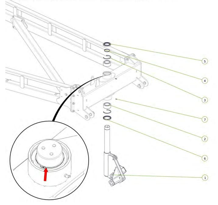
Circlip fitted to jockey wheel shaft
