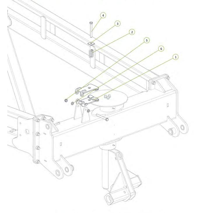
Check tension of brake caliper spring (50-63mm road transport)
