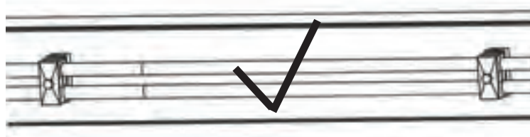
Correct layout of hoses
