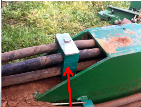
Extra stack clamp added to mount extra main lines to existing main lines
