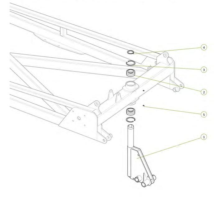
Circlip fitted to jockey Wheel shaft
