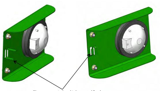
Please ensure to bend tabs up and feed wire through, so the light cable is secure
