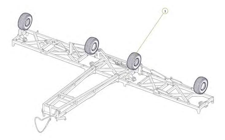
All wheel nuts tightened to 100fl-lb / 140Nm
