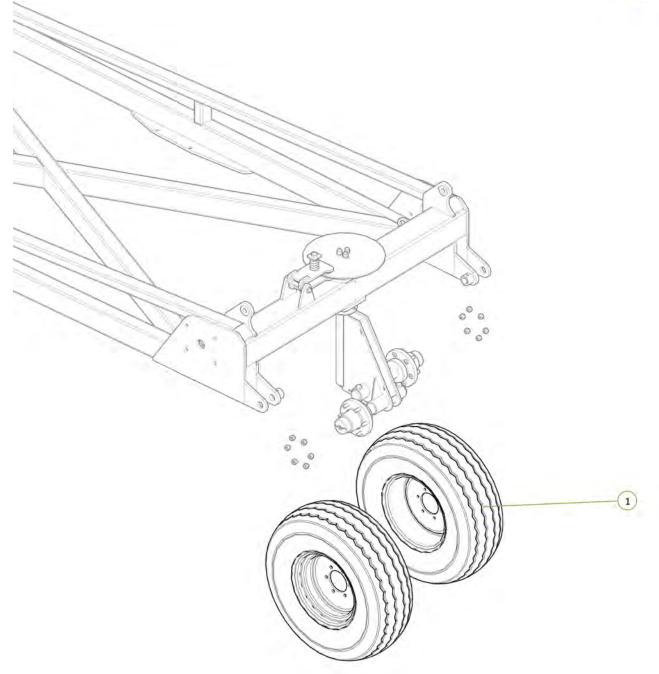
All wheel nuts tightened to 90ft-lb / 125nm
