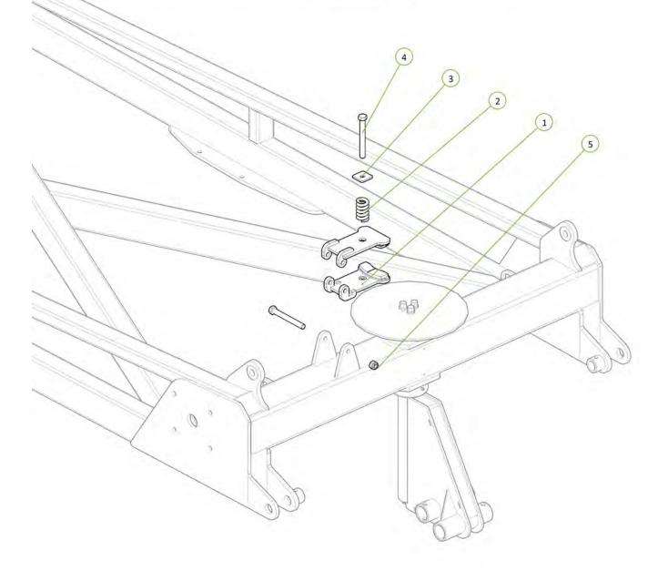
Check tension of brake caliper spring (50-63mm road transport)
