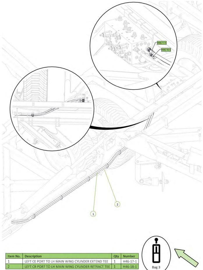
LEFT CR PORT TO LH MAIN WING CYLINDER RETRACT TEE H46-18-1 1
