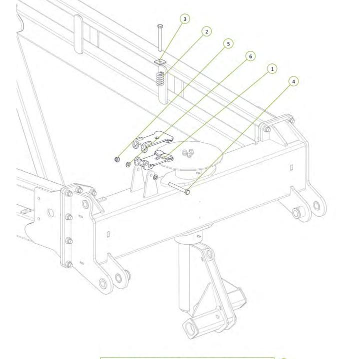
Check tension of brake caliper spring (50-63mm road transport)
