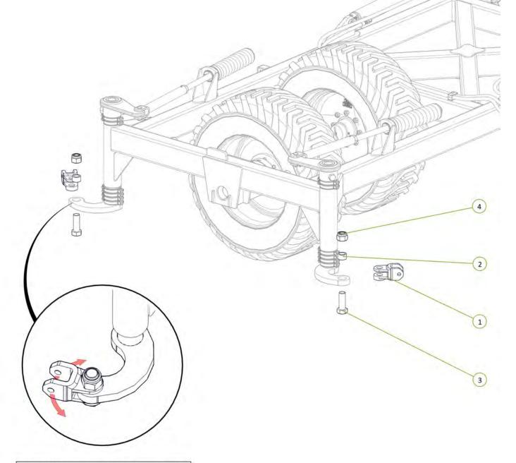
Ensure ALL clevis's can pivot after installation
