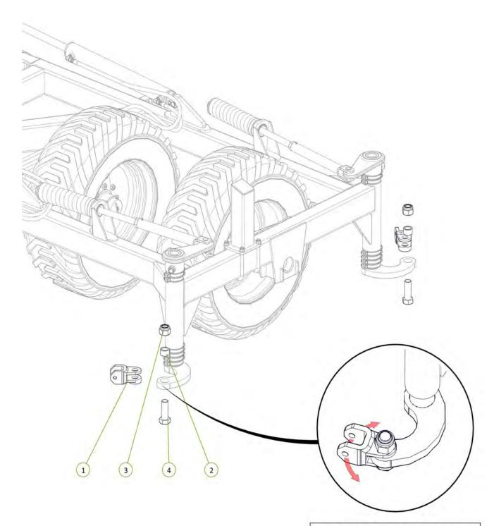
Ensure ALL clevis's can pivot after installation
