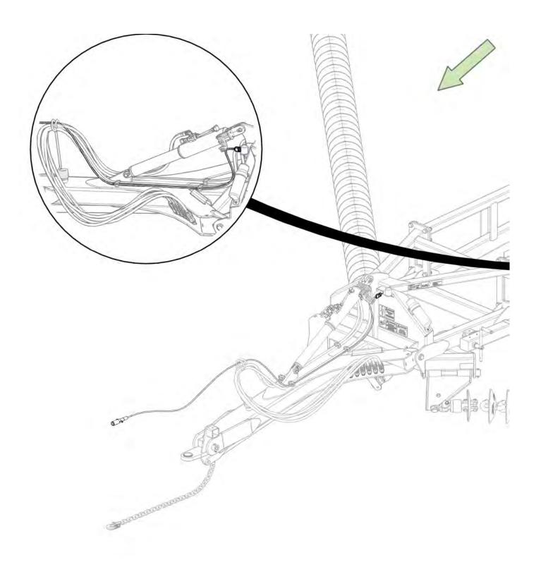
Where required secure loom to hydraulic hoses or tabs provided
