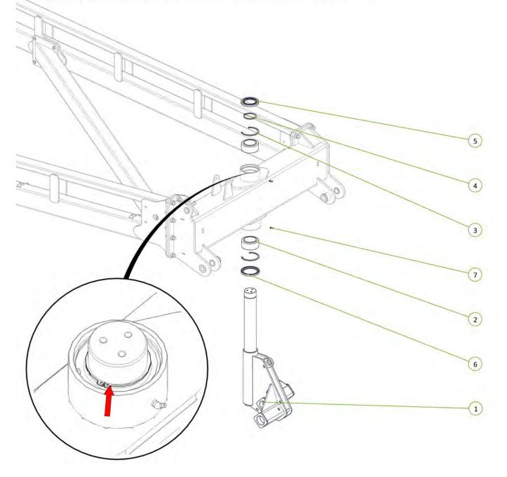
Circlip fitted to jockey wheel shaft
