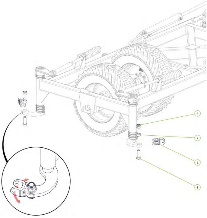
Ensure ALL clevis's can pivot after installation
