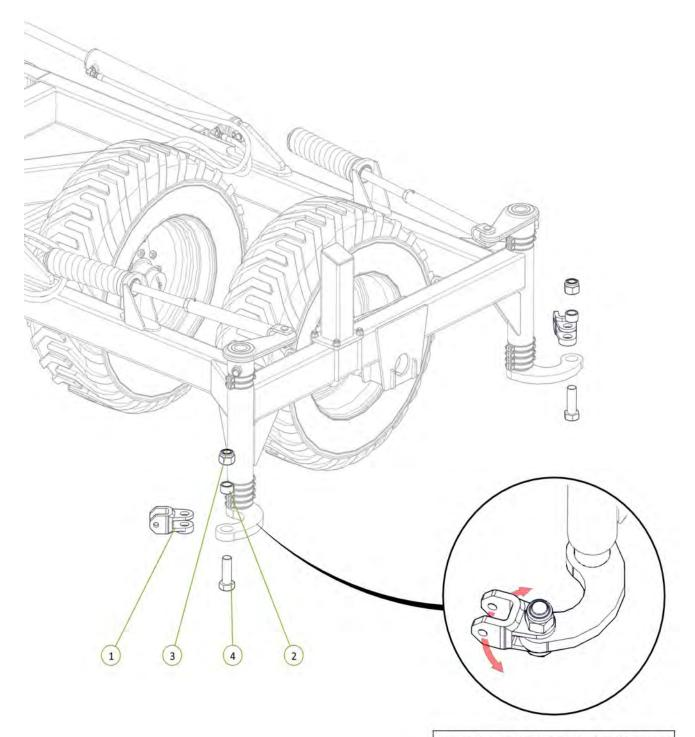
Ensure ALL clevis's can pivot after installation
