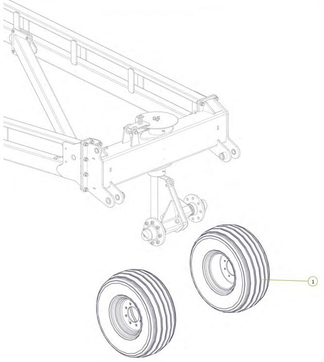
All wheel nuts tightened to 100ft-lb / 140Nm
