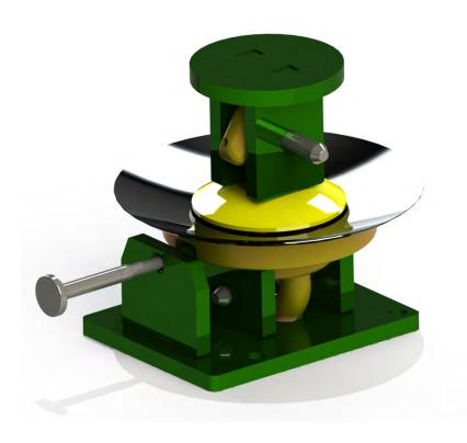
Figure 3: CL2 disc with press jig in Closed position
