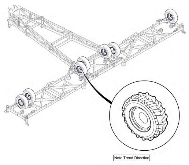
All Wheel nuts tightened to 265ft-lb / 360Nm
