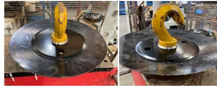
13. Align the hook so the locating hole in the shank is aligned with the pin hole in the eye clamp casting.
